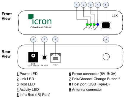
\* IR port used to pair the LEX unit and the REX unit only
